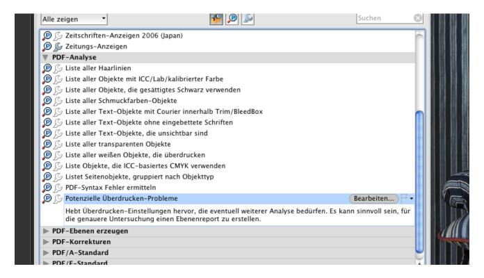
Advanced - Preflight ... - PDF analysis - Potential overprint problems - double click (German in this photo: "PDF-Analyse" - "Potenzielle Überdrucken-Probleme")
