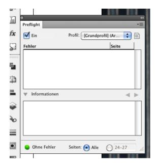
the wrong profile (standard -German in this photo: "Grundprofil") does not discover the error and does not warn you
